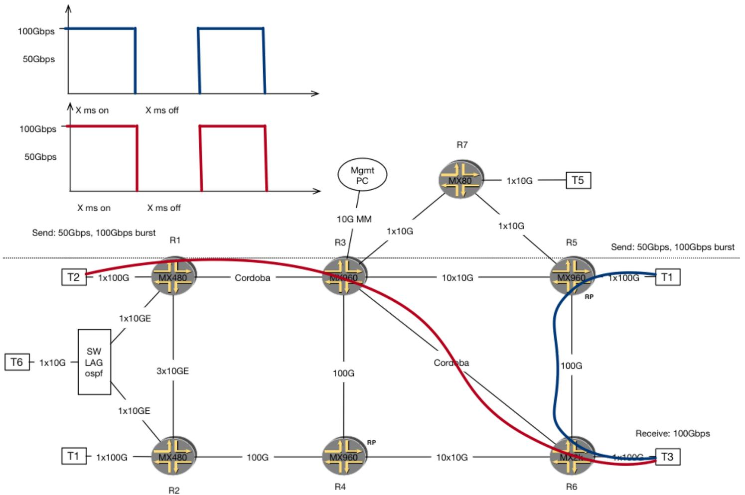
T2 sends traffic towards T3 at 100Gbps, to verify lowest packet size without dropping packets. Use that packet size for the rest of the test.
